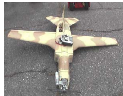
Figure 6. Mig 117 Bravo modified target drones were equipped with modern engine and Micro-Pilot autopilot
