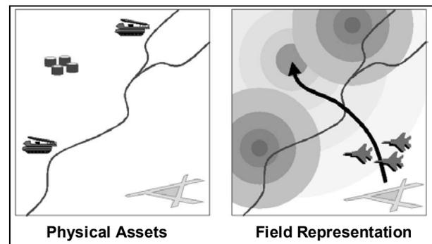
**Figure 1: Potential Fields Corresponding to Physical Assets**
